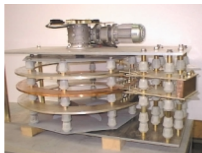
(reduced scale slip ring, made as show case on a larger project order)
