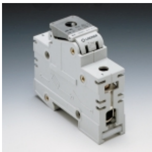
DO LINOCUR Switch-disconnector for construction ~ 440 V, D02 sealable, with snap-on mounting for top-hat rails as per DIN EN 50022
